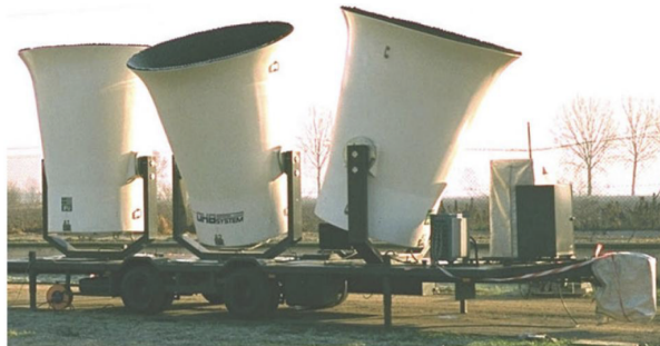
Figure 1.4: A three antenna SODAR for wind and turbulence profile measurements up to 1000 m above ground. Figure adapted from [4].
